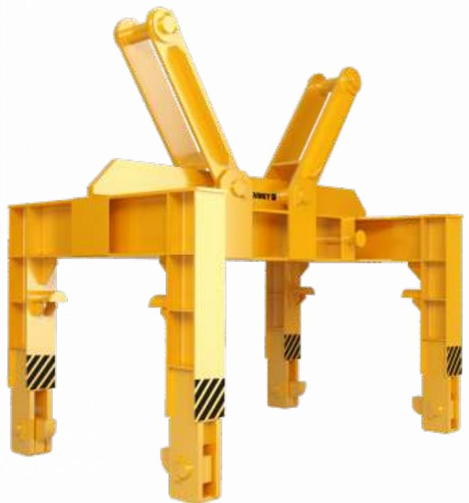
**DIMET spatial beam** for handling mill rolls consist of a welded housing with side plates for cargo suspension, which rotate around the axis. Depending on the crane capacity, the beam can be equipped with a suspension for a single or double hook.
