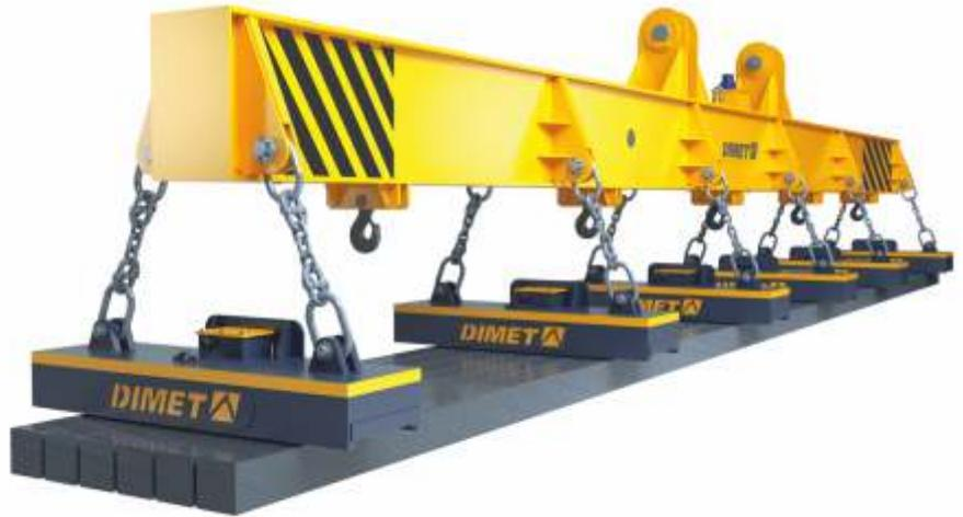
**A series of magnetic beams** is designed for handling long square blanks, blooms and other types of rolled products of similar geometry. We recommend the use of magnetic beams for handling square and rectangular long loads with specially designed DIMET electromagnets from the EMG and EMGS lines.
